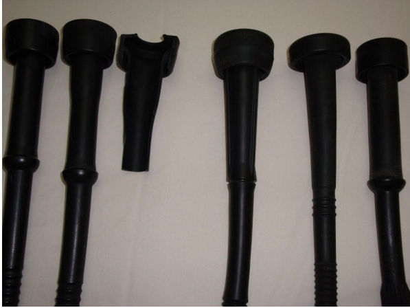
Figure 2: CMS new, CMS end of life, CMS end of life section, three conventional at end of life
