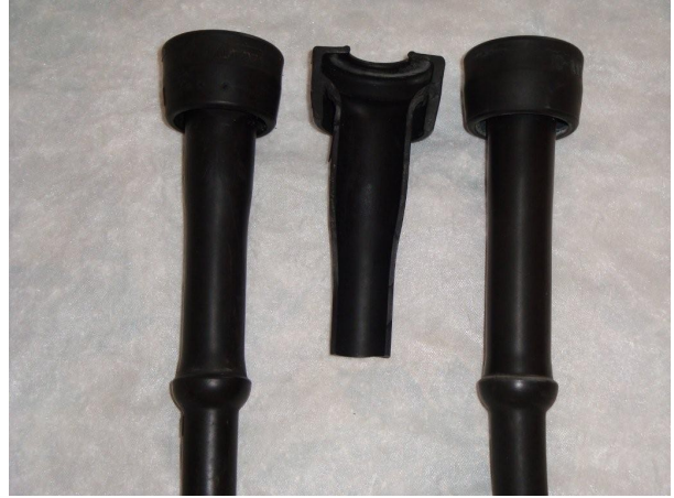
Figure 3: CMS end of life, CMS end of life sectioned, CMS end of life used with conventional pulsation
